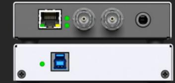
The accompanying software package comprises an AVDECC controller, which provides essential functions to discover all AVB devices in a network and manage connections of incoming and outgoing streams. An additional headphone output allows high quality monitoring.
